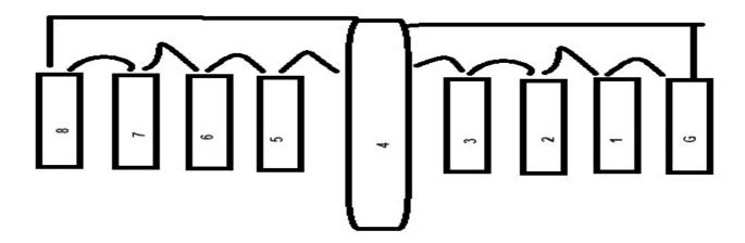
To ensure seamless interconnectivity across floors and reliable connectivity with the IT Room, a 24-core Multimode Optical Fiber should be deployed from each floor to the fourth floor, where the data center is located. For every connection leading to the IT Room, Multimode SFPs will be utilized to maintain optimal performance and compatibility.
